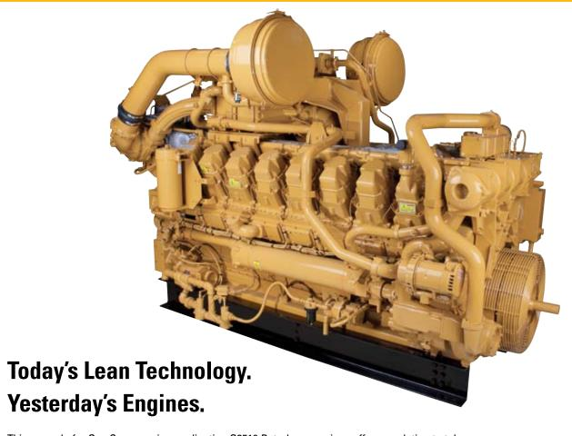
This upgrade for Gas Compression application G3516 Petroleum engines offers a solution to take your existing engine and upgrade to ULB technology. This latest proven technology utilizes state of the art ADEM III technology, Mass Flow Air Fuel Ratio Control, and NOx sensors to operate at not-to-exceed 0.5 or 1.0 g/bHp-Hr levels with higher altitude capability throughout the total speed range.
